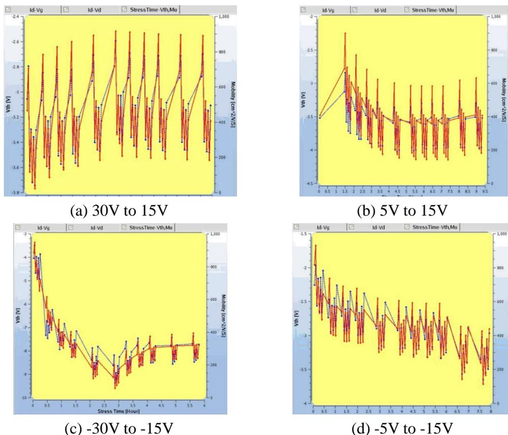
Figure 5:  $V_{th}$  shift vs. time for different stress sequence
