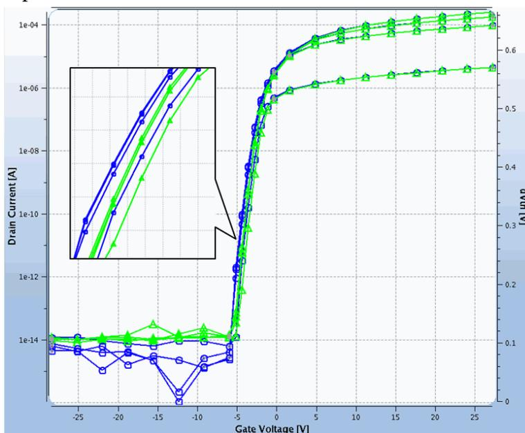
Figure 1: Initial  $I_D$ - $V_G$  Measure with Various  $V_{DS}$  Bias
