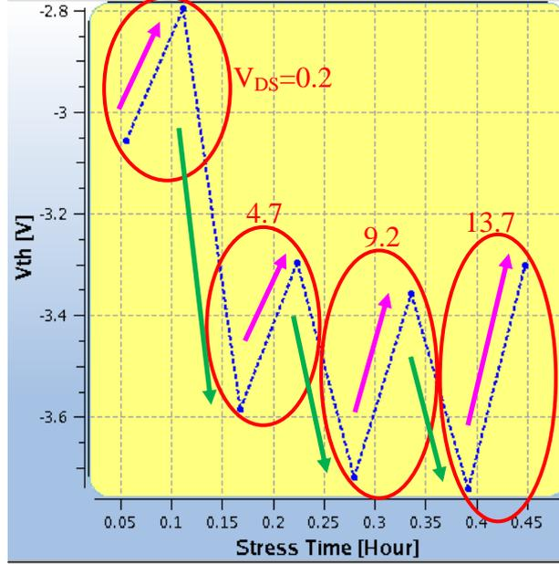
Figure 2:  $V_{th}$  plot in a set of  $I_D$ - $V_G$  measure
