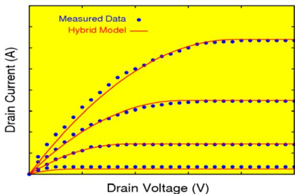
Fig. 1: MSIM extracted model and measured data comparison of  $I_{DS}$  versus  $V_{DS}$  at various  $V_{GS}$  for a-IGZO TFT device
