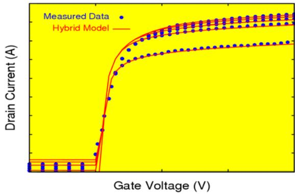
Fig. 2: MSIM extracted model and measured data comparison of  $I_{DS}$  versus  $V_{GS}$  at various  $V_{DS}$  for a-IGZO TFT device
